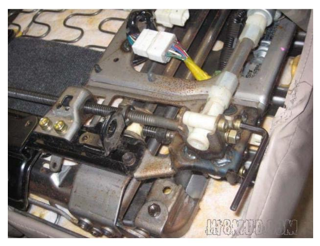
4) To take off the shaft bolts, hold the shaft with a vice grip. Remove the little plastic the rear supports, then unscrew the gear housing. When you remove the shafts from the slides of the seat, do your best not to allow the thing to twist at all, and thus change position. It's important that both sides are at the same position, in relation to each other, or it's going to try to push your seat crooked and probably not work too well.
