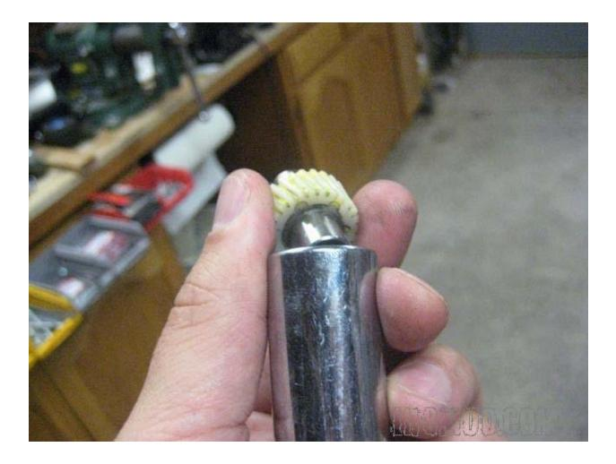
6) Now notice how there are three little indents (in the picture in the post above) in the side of the stock gear, where the thing has been staked in place. When removing, press it so that it doesn't make those stakes pass over the knurls of the shaft.
