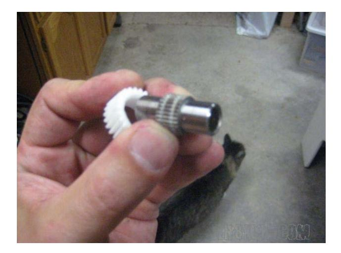
To press it on you can use a smaller socket if you want, and actually that will help create a stop when it smacks against the raised knurled portion of the shaft. Once on, remove the little chips the knurls made with a utility knife. You can see by the material removed how well engaged the knurls of the shaft must be with the new gear. Then it's just bolt it all back up, put the rubber washers in the same orientation as how they came out, and put a mess of grease around the new gear teeth.
