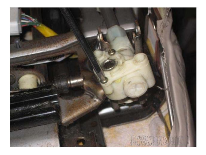
5) Notice how there's a thick rubber washer on the "inside" of the shaft, and a thin one on the "outside," against the little panel you just took off. Make sure to put them back in the same orientation when reassembling.
